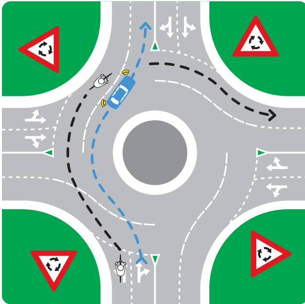
Bicycle at a roundabout turning right from left lane.
