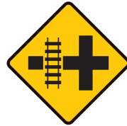
Level crossing on side road.
